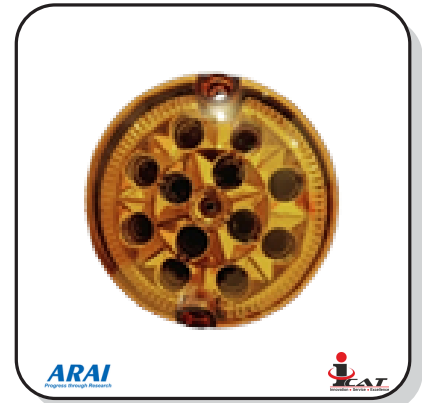
LED FRONT & REAR DIRECTION INDICATOR ASSY 12 LED Part No. VAI-080
